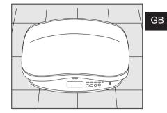
Level gauge Check • Place the scale on a flat surface to ensure accurate measurement. • Turn the four adjusters such that the air bub-10000 ble in the level guide is positioned exactly in the center. Confirm that all four adjusters are in contact with the surface. Level gauge <View from above> Red  $\diamond$ Air bubble Adjusters (4)
